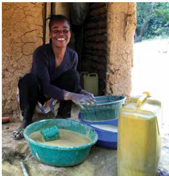
A mining team leader—who leads a team of four male miners—uses Just Gold sieves to wash pulverized ore.
