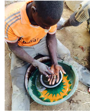
An artisanal miner uses mercury for the process of amalgamation and cyanidation of gold at a mine near Gaoua, Burkina Faso.
